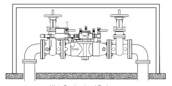
WattsBox Insulated Enclosures Available in Aluminum or Fiberglass. For more information, send for ES-WB.
