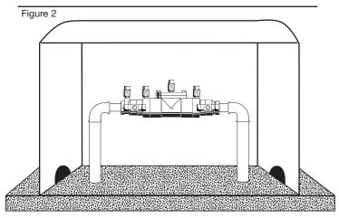
WattsBox Insulated Enclosure Available in Aluminum or Fiberglass. For more information, send for ES-WB.
